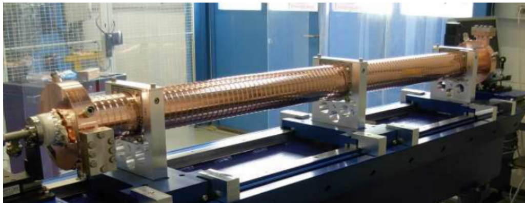
Figure 1.10: Picture of a C-band 2 m-long (113 cells) accelerating structure for the SwissFEL facility, operating in TW 2\pi/3 mode at 5.7 GHz and 28 MV/m gradient.
