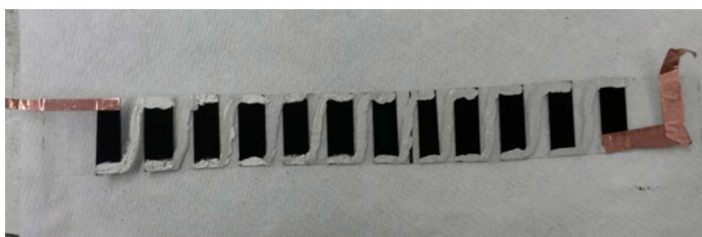
Figure 6.16 Pictures of: (a) 20 BL of MWCNTs/MWCNTs after PEDOT polymerization and (b) fundamental unit of thermoelectric module.
