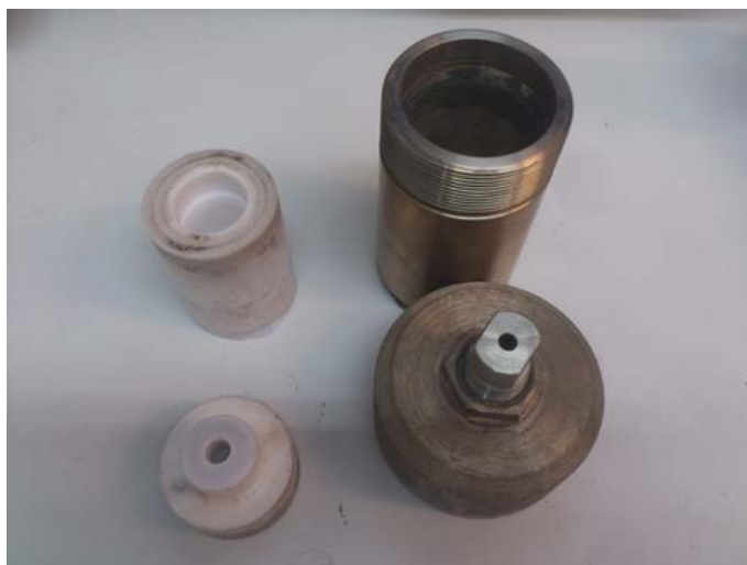
Figure 4.8 Photograph of a Teflon autoclave with its steel holder .
