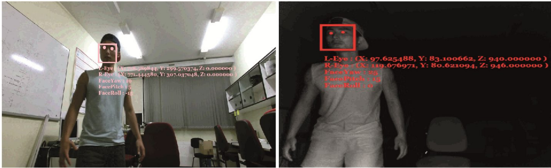
Figure 4 The Kinect 2 is a device that permits to track the 3D position of an observer. It uses infrared technology, so it works in dark environments.
