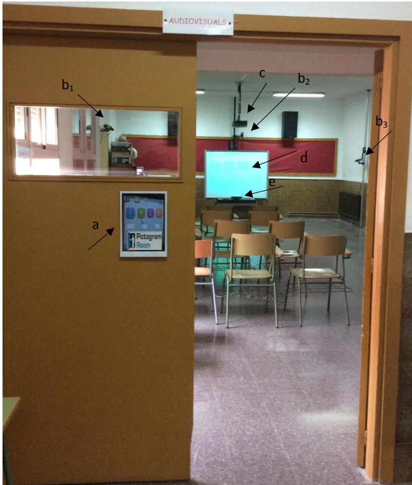
Figure 13. Room arrangement: (a) board for the pupils to place the PECS cards, ( b_{1,2,3} ) video cameras, (c) projector, (d) IDW, and (e) Kinect.
