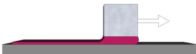
Fig. 2 Schematic of the meniscus coating technique employed.
