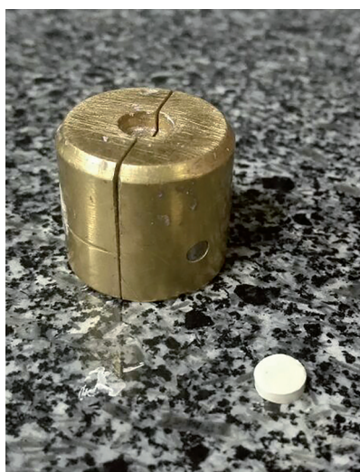
Fig. 1. Split mold and specimen.
