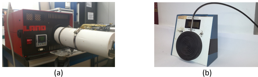
Figure 4.6. Sources (black body) of calibration used for: (a) direct indoor calibration – LAND P80P – and (b) direct outdoor calibration performed with platinum thermometer.
