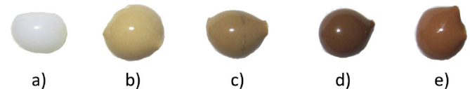
Fig. 10. Photograph of colored glazes obtained from mixtures of the nano-pigment \text{Cr}_{0.15}\text{Sb}_{0.15}\text{Ti}_{0.7}\text{O}_2 , without and with annealing at different temperatures, and a standard frit: a) frit without nano-pigment; b) with as-precipitated nano-pigment; c) with nano-pigment annealed at 800 °C; d) with nano-pigment annealed at 1000 °C; e) with nano-pigment annealed at 1200 °C.
