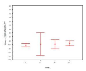
**Fig. 3a,b,c,d.** Error Bar Graph for each group: Results of Deflex compared with A,H and VLC for  $\Delta E$  (colour change), sorption, solubility, surface hardness.
