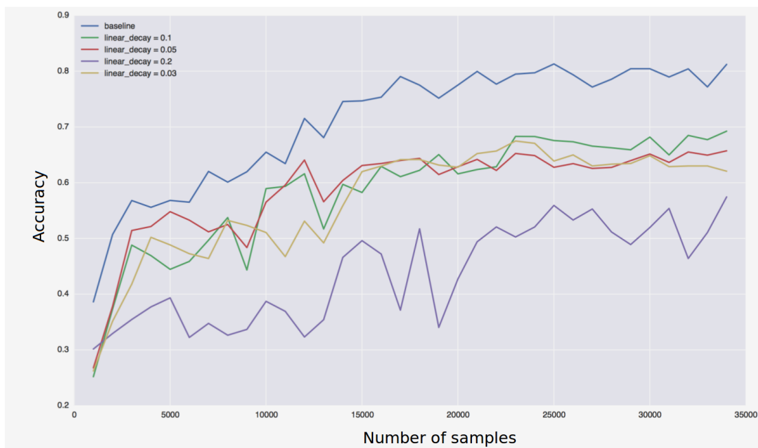
FIGURE 4.14: evtCD RBM with simplified LIF neuron learning curve for different membrane decay constant.
