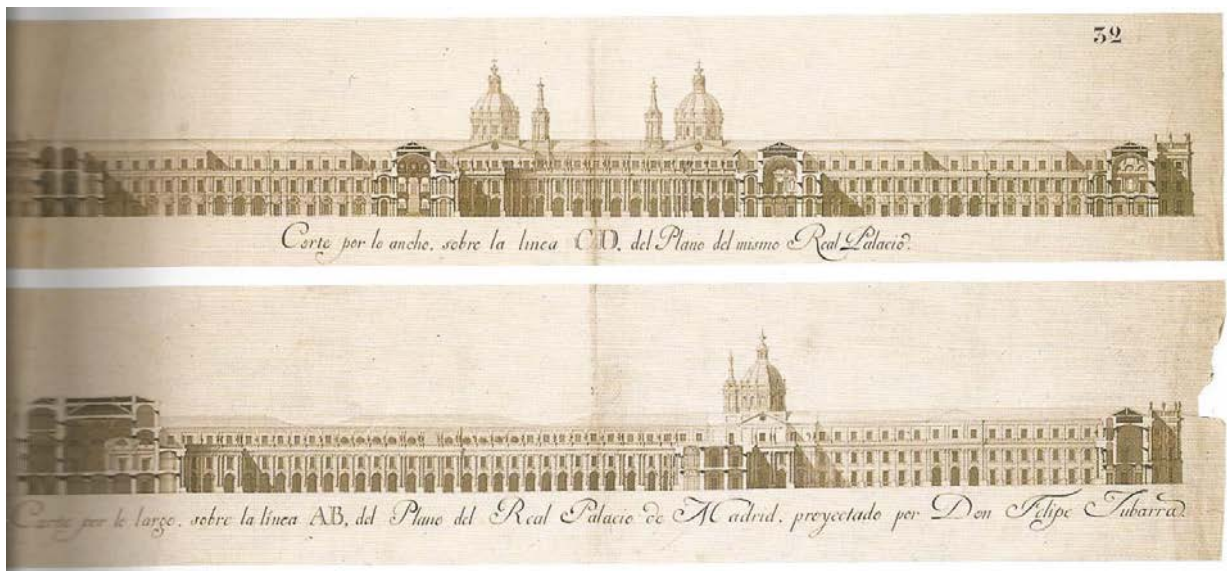
Fig. 200: Intersection on the line CD of the same Royal Palace, Intersection on the line AB of the plan for the Royal Palace of Madrid, designed by Don Felipe Juvorra
