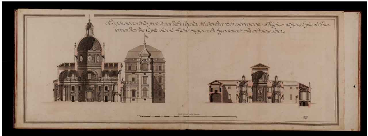
Fig. 30: Internal profile of the right part of the church, the belvedere seen from the exterior and the old pavilion, section of the ground floor of the two lateral chapels of the main altar and apartments
