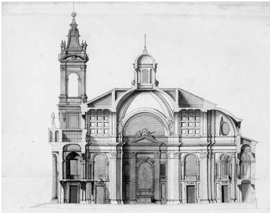
Fig. 44: F. Juvarra. Longitudinal section to southeast according to the first project, not realized, of the façade of the church of St. Uberto at Venaria Reale
