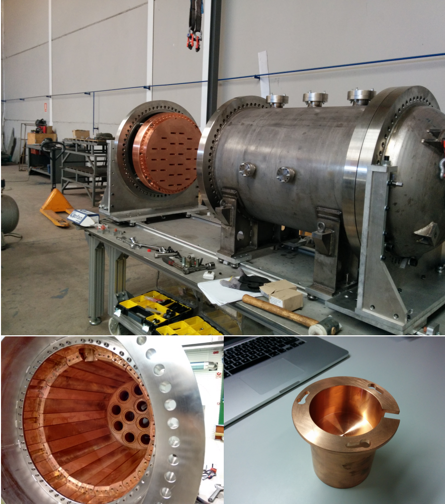
Figure 4.9: (Top) The vessel with the TP endcap opened showing the TP copper shielding. Copper bars barrel screwed on the inner vessel thread (bottom left) and the copper top-hat extra shielding (bottom right).
