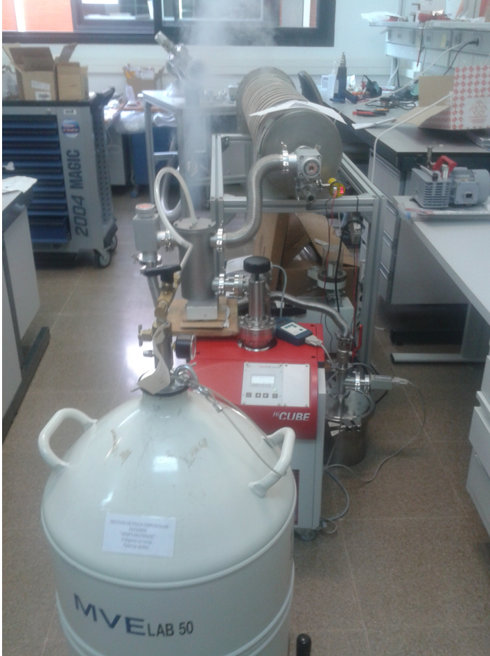
Figure 4: The ArDM chamber used for TPB deposition located at IFIC. The chamber is in the background with the vacuum turbo-cube in the foreground. The chamber is being evacuated through a liquid nitrogen cooled cold trap to protect the turbo pump from TPB contamination.
