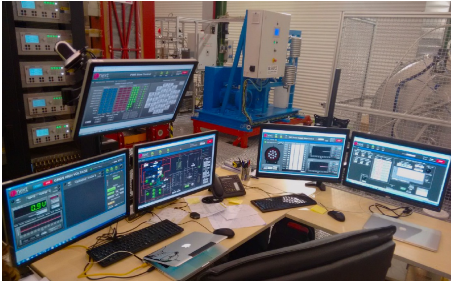
Figure 4.14: Slow control displays showing the monitor and controls for the gas system, HHV, sensors and electronics.
