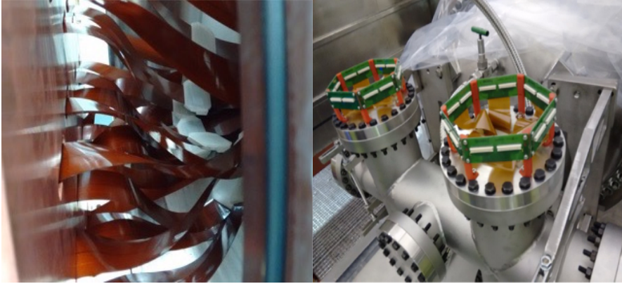
Figure 4.8: (Left) KDB end-tail connected through the copper shielding plate to the FFC towards the FR4 feedthroughs and adapter boards (right).
