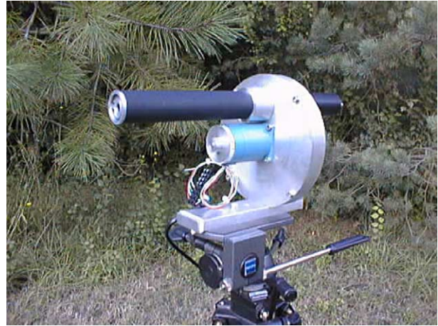
Fig. 2. Photograph of the Passive Multi-Wavelength Fluorescence Detector (PMFD).
