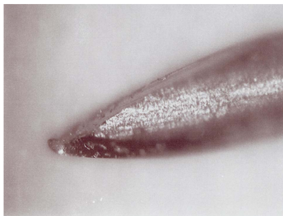
Fig. 1. Monoprotect® needle with non-preserved bevel after truncal block of the inferior alveolar nerve (100X).
