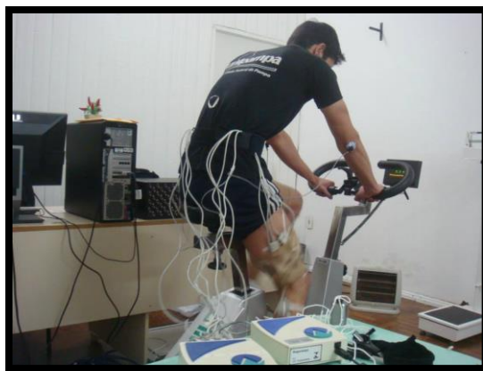
Figure 3.10. Surface electromyography measurement during cycling.
