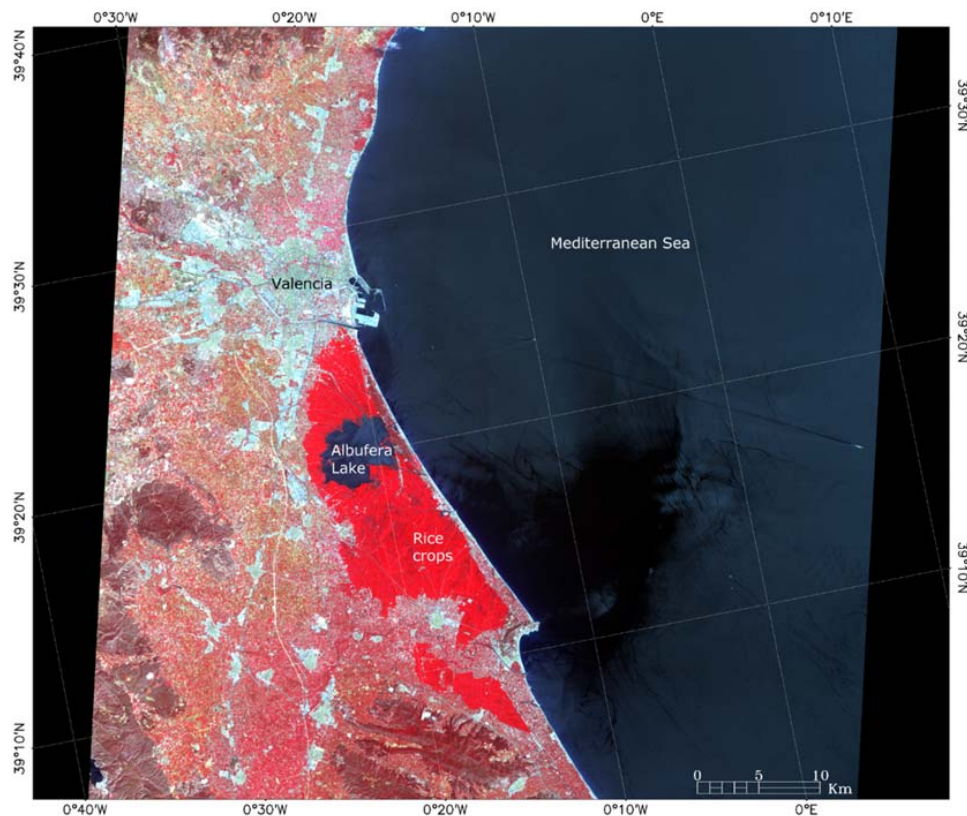
Figure 1. Scene over the study area on 3 August 2004 using VNIR ASTER Channels 3n ( 0.81 \mu\text{m} ), 2 ( 0.66 \mu\text{m} ) and 1 ( 0.56 \mu\text{m} ) to compose the RGB image, respectively.
