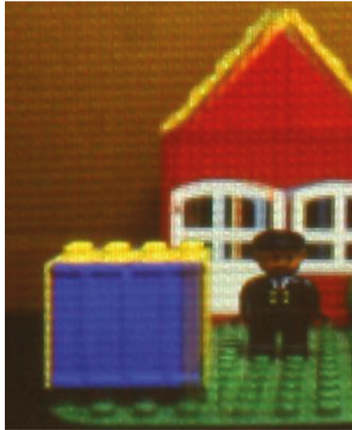
Fig. 2.- The crosstalk causes a distortion on the image perceived by the observer. On this image, the crosstalk can be seen on the roof and the door of the house and, also, on the right side of the block situated at the front of the scene.
