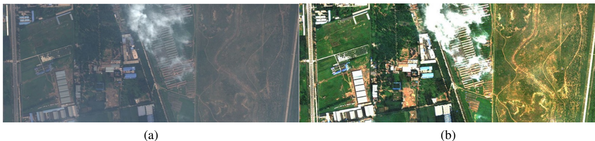
FIGURE 3.4.5: RGB from Landsat 8 over Naples, Italy, before (a) and after (b) the application of the Acomp atmospheric correction algorithm. Source DigitalGlobe's GBDX platform.
