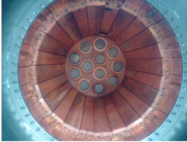
Figure 3.14: Detailed view of copper bars shielding the vessel body, with the energy plane viewed from the anode.
