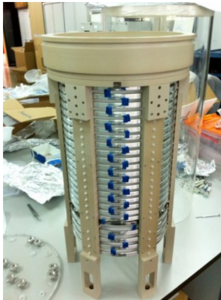
Figure 3.5: Cross-section drawing of the NEXT-DEMO prototype with major parts labelled (top), and image of the field cage standing on the lab (bottom).
