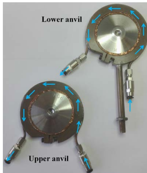
Figure 3.7: Home-made water cooling system. Blue arrows indicate the water flow.
