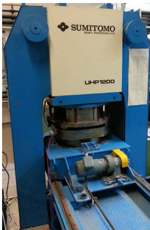
Figure 3.23: Sumitomo 1200 tons multi-anvil press.
