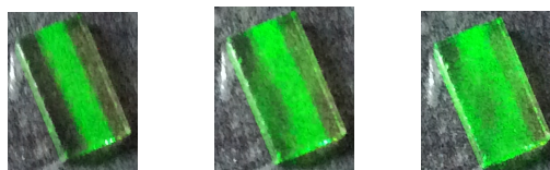
Fig.10. Energy transfer (beam fanning) in a non- degenerate four wave mixing configuration. The three images capture instants separated by 10 sec.
