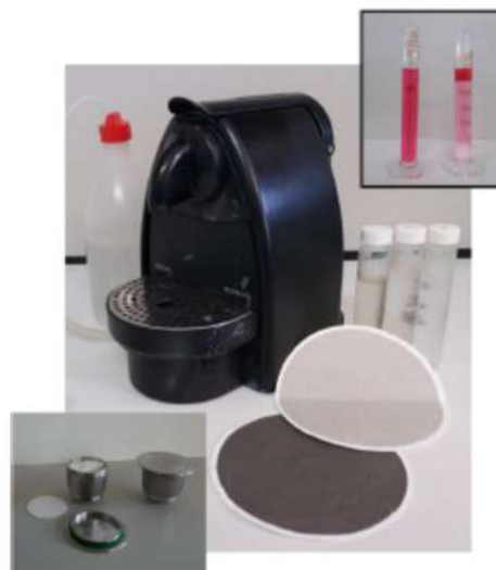
Fig. 1. PM10 filters, hard cap espresso machine, and stainless steel reusable caps employed in this study. Inset: Detail of the salting-out effect using a colouring agent for identification purposes.
