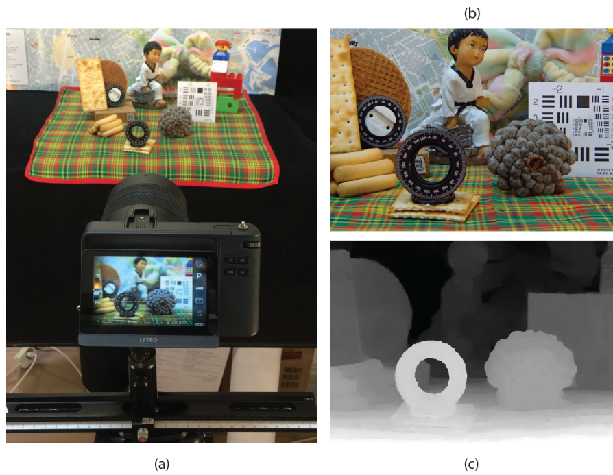
Figure 6. (a) Experimental set-up of the real capture of the 3D scene. (b) The RGB image extracted from Lytro Desktop software. (c) The depth map of the scene extracted from Lytro Desktop software.
