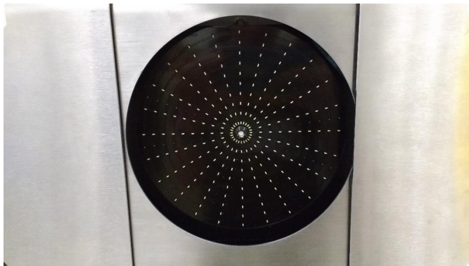
Figure 3.4. Light Disturbance Analyser instrument and the distribution of the central and peripheral light sources.
