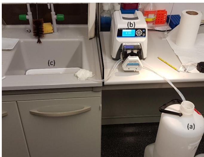
Figure 14. Decellularization setup. The selected perfusion media are pushed from the containers (a) through a peristaltic pump (b) into the organ with cannulated arteries. The organs are submerged in a deep tray, cells are lysed, and cellular material is removed through the perfusion with the DC medium, the exiting medium overflows from the tray into the sink (c).
