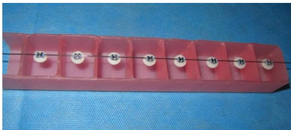
Fig. 2: Wax boxes with wire ratchet for mounting the disks.
