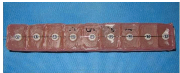
Fig. 3: Mounted disks for bracket bond strength testing.
