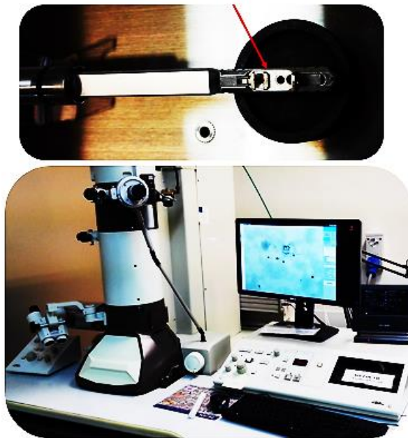
Figure 21. Transmission electron microscopy. Preparing the sample and mounting it (red arrow) in the holder (upper image). Transmission electron microscopy (bottom image).
