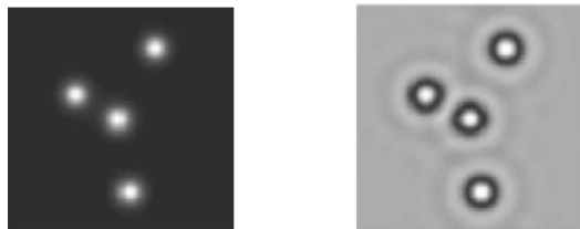
Figure 1.4: Bright amplitude (left) and dark-ring (right) cavity solitons in a DOPO. From [29].
