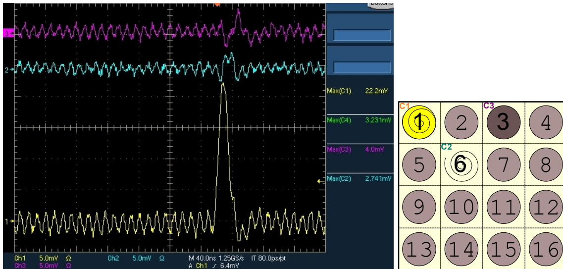
Figure 18: Channel 1: signal from the illuminated and plaited SiPM (Nr. 1), Channel 2: signal from the plaited SiPM (6). Channel 3: signal from the non plaited one (3). Nr. 6 is removed and Nr. 3 covered.
