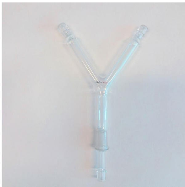
Figure C2. Y-tube olfactometer used in the experimental bioassays (Vidrafoc ®, Valencia Spain). The tube inner diameter was 1.5 cm, the basal branch was 8 cm long and each of the Y-branches 6 cm long. Compressed air entered at a constant flow rate through a glass flask with activated charcoal connected with a second flask with distilled water. Teflon tubes were used to connect the system (Labbox, Barcelona Spain).
