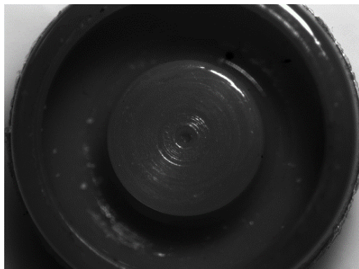
Fig. 3: Photomicrograph of the unused Locator attachment retentive male insert.
