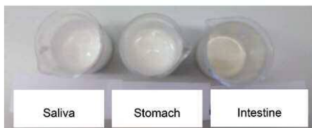
Figure 2. Visual appearance of the fresh methylcellulose O/W emulsion and after in vitro digestion at 37 °C.
