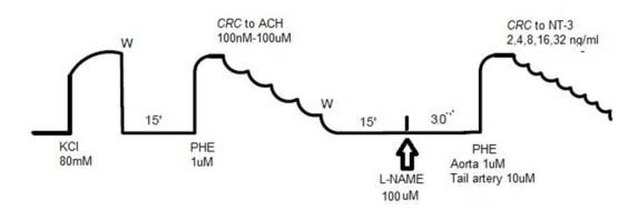
**Scheme 1.** Schematic drawing showing the experimental procedure used in rat vessels to study the role of NT-3 on vascular tone in the presence or absence of L-NAME. PHE: Phenylephrine, ACH: Acetylcholine. CRC: concentration response curves, W: washing.
