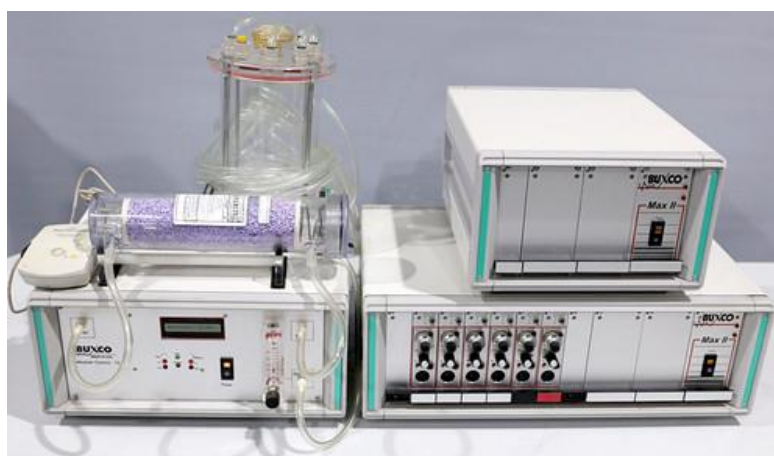
Figure 21. Buxco Small Animal Whole Body Plethysmography apparatus.
