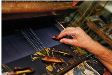
Fig. 1. Making a Valencian espolin with a Jacquard loom. It can be seen how the golden threads do not go from side to side of the fabric, but remain concentrated around the pictorial motifs.
