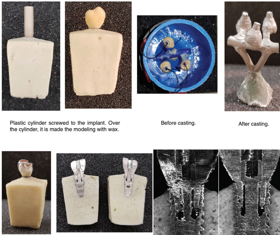
Model after being sectioned in half with a diamond saw and its picture with the stereomicroscope. Fig. 1: Study procedure example.
