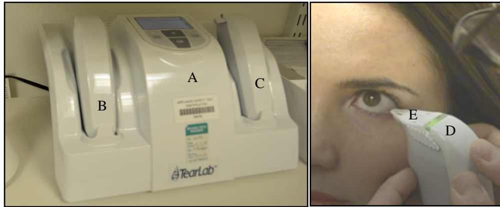
Figure 22 TearLab® Osmolarity System (A) with the Osmolarity Test pens (B and C) and during the collection (D) of a sample of tear film through the Osmolarity Test card (E).
