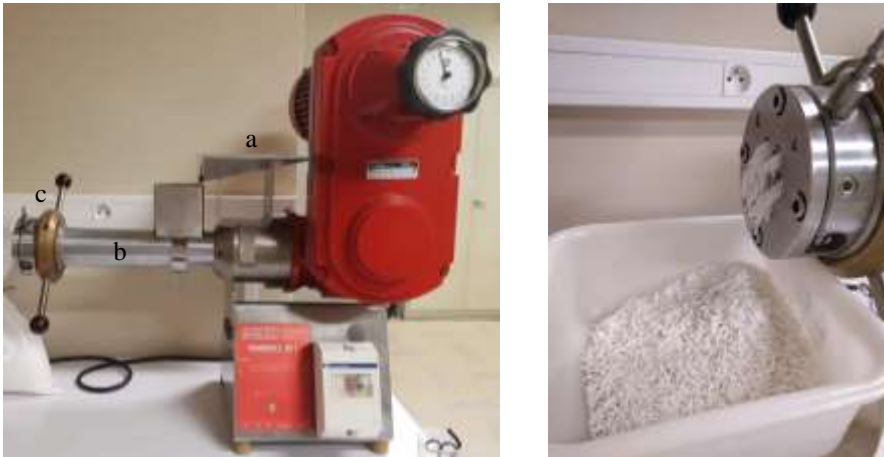
Figure 8. Example of a extruder (left) with the hooper or feeding zone (a), followed by the barrel with a screw and the drying zone (c) through which the MCC extrudates are obtained (right).
