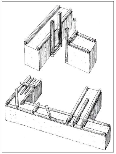
**Figure II.3**: Wooden reinforcement of the rubble walls at Akrotiri, Thera. Palyvou 1999, Fig. 17.
