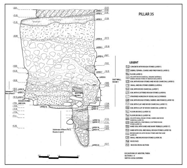
**Figure II.8**: Cross-section of Pillar 35 – Section A-A'. Courtesy of the Archaeological Society in Athens, Excavations at Thera.
