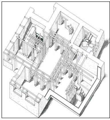
**Figure II.6**: Representation of the ground level of Rooms 1 to 8 at Xeste 3, where the wooden infrastructure of the pierand-door partitions is shown. Palyvou 1999, Fig. 192.
