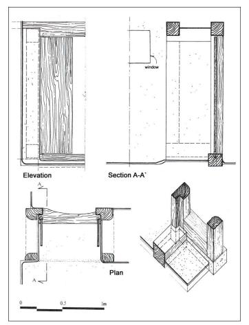
The openings for the buildings, doors, and windows were constructed in more or less the same way (Fig. II.5). The wooden framework of the jambs of the doors was made of two pairs of posts resting on transverse beams, while two more transverse beams were placed on top of them to hold them all together. The lintel was formed with two or more horizontal beams. The whole structure was held secure in the wall, as it was attached to the wooden grid. The only difference between interior and exterior
