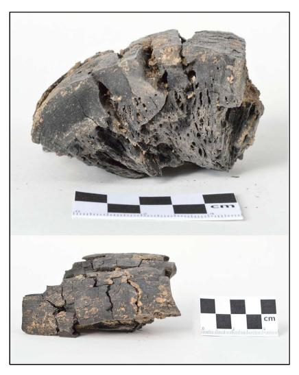
**Figure V.15:** Part of a wooden beam recovered from Room 6 of Xeste 3 (sample  $\Delta$ 5).
