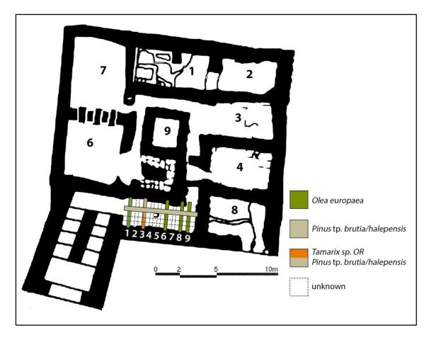
**Figure V.28:** Reconstruction of the beams supporting the upper floor of Room 5 of the House of the Ladies, based on anthracological and architectural evidence.
