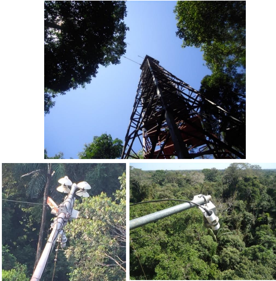
Figure 4.9. Tambopata test site tower site (perspective from below) together with images of CNR4 net radiometer (lower left) and infrared radiometers (lower right).
