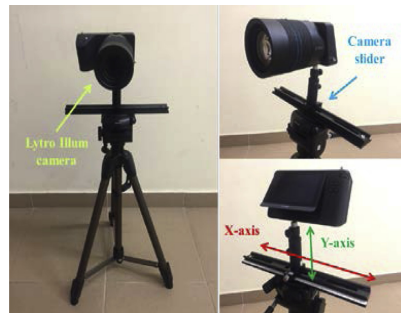
Fig. 3. Proposed stereo-plenoptic camera system.
