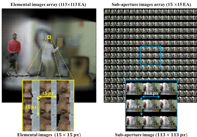
Figure 2.4: Conversion example between the elemental images array and the sub-aperture images array. Left integral image contains 113 \times 113 elemental images (with 15 \times 15 pixels each), and the right array contains 15 \times 15 sub-aperture images (with 113 \times 113 pixels each). But, both images have same size ( 1695 \times 1695 pixels).
