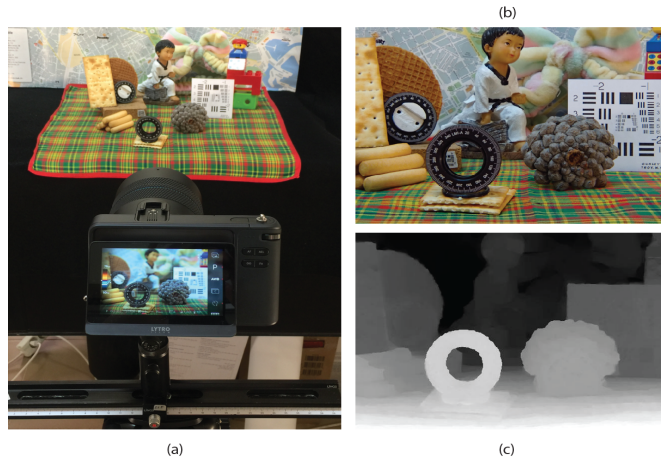
Figure 6. (a) Experimental set-up of the real capture of the 3D scene. (b) The RGB image extracted from Lytro Desktop software. (c) The depth map of the scene extracted from Lytro Desktop software.
