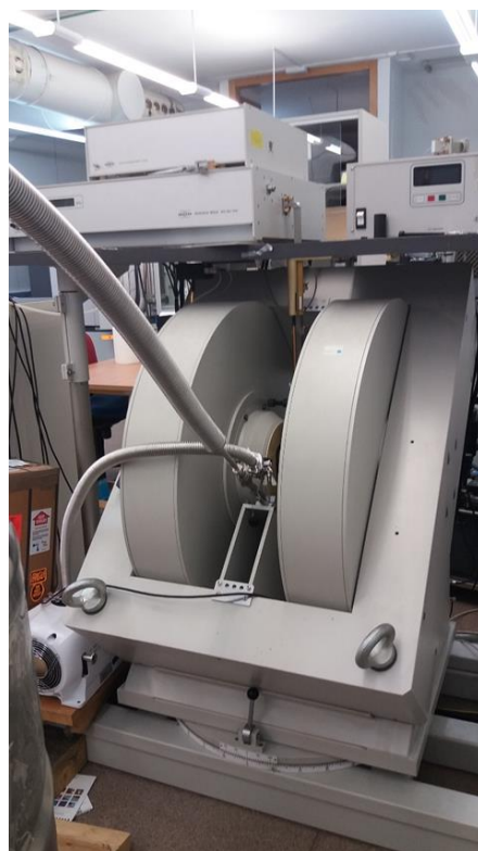
Fig. 5 Basic picture of a standard EPR spectrometer. Note the two parallel coils and the thick pipeline carrying liquid helium to the cavity.
