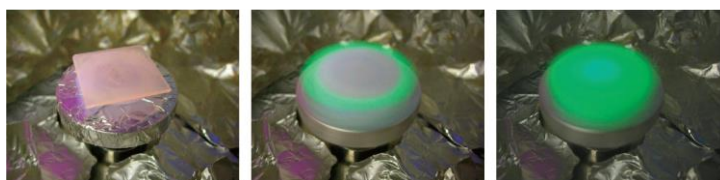
Figure 1.1. Pictures of in situ synthesis of luminescent perovskite nanostructures under UV light. Perovskite precursor solution (left) is uniformly dropped onto a mesoporous alumina thin film. During spin-coating, the quick vaporization of the organic solvent triggers the crystallization of highly luminescent lead bromide perovskite nanostructures within the mesoporous alumina. Adapted from reference 25.
