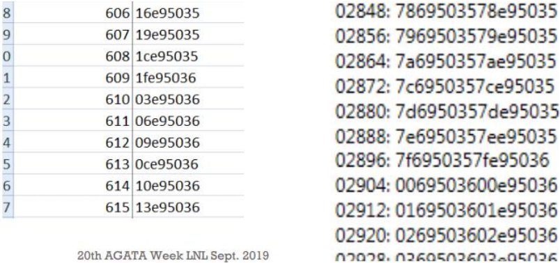
Fig. 6.17. The results of the first Proof-of-Concept, for the data writing test, presented on AGATA Week 2019. The left side is the data written to disk at the server. The right side is the data sent from the PACE prototype SOM and is a 28-bit sample.
