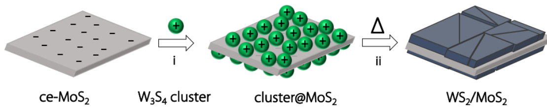
Scheme 1. Pictorial representation of WS_2/MoS_2 synthesis: (i) Synthesis of cluster@MoS_2 ; (ii) Calcination of cluster@MoS_2 to give rise to the final WS_2/MoS_2 heterostructure.
