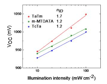
**Figure 3.** Light intensity dependent  $V_{oc}$  and extracted ideality factors for perovskite solar cells with different HTMs.
