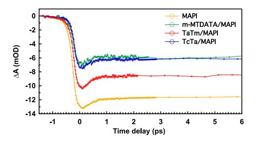
**Figure 4**. Time-resolved transient absorption dynamics for neat MAPI and the perovskite/HTM double layers, excited at 600 nm (at constant excitation density of  $1.4 \cdot 10^{17}$  cm<sup>-3</sup>) and probed at the perovskite maximum ground state bleaching band.
