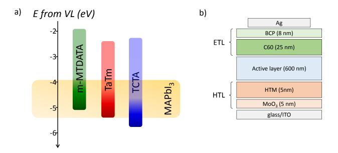
**Figure 1.** a) Energy diagram of different HTMs with respect to MAPI. The energy values of the HOMOs were determined by photoemission spectroscopy in air (PESA) (see supporting Information Figure S1). b) Scheme of completed stack with different HTMs.
