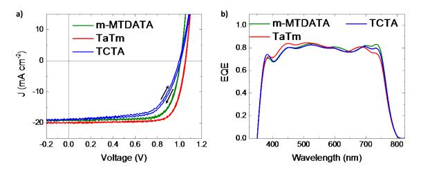
**Figure 2.** (a) J-V curves under 100mW cm<sup>-2</sup> illumination in forward and reverse bias and (b) EQE spectra of representative perovskite solar cells produced with different 5nm thick HTMs.
