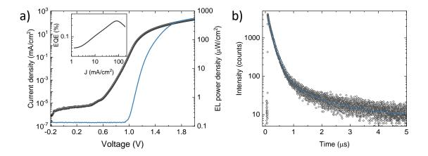
**Figure 3.** a) Current density (symbols) and electroluminescence power density (line) vs. the applied voltage for a MAPbI<sub>3-x</sub>Cl<sub>x</sub> perovskite diode. Inset shows the EQE for
