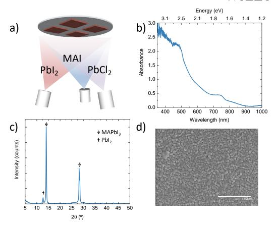
**Figure 1.** a) Schematics of the three-source vacuum deposition of  $MAPbI_{3-x}Cl_x$  thin films. Characterization of perovskite films: b) absorption spectrum, c) XRD pattern and d) SEM image of the sample surface.
