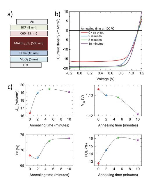
**Figure 2.** a) Scheme of the vacuum deposited perovskite diode and b) its electrical characterization for different perovskite annealing temperatures; J-V curve under simulated solar illumination are reported in forward (from short to open circuit, solid lines) and in reverse (from open to short circuit, dots) scan. c) Summary of the photovoltaic parameters as a function of the annealing time at 100 °C.
