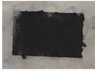
Figure C.7: Photograph of \text{Cs}_2\text{SnI}_6 powder – exposed to air – fixed on adhesive tape on a glass substrate.
