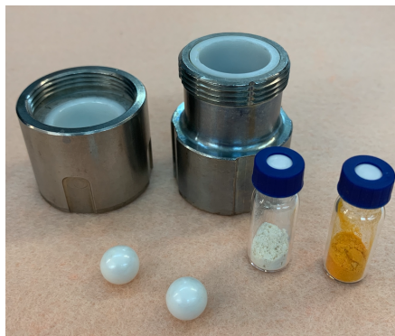
Figure 1.6: Photograph of a ball-mill jar and two zirconia beads used for the mechanochemical synthesis of multinary metal halide semiconductors. The left vial contains the pristine perovskite precursors ( \text{CsBr} and \text{PbBr}_2 ). The right vial contains the \text{CsPbBr}_3 perovskite that has been formed by ball-milling of the stoichiometric perovskite precursors. See Chapter 2 for a detailed description about the experimental methodology.
