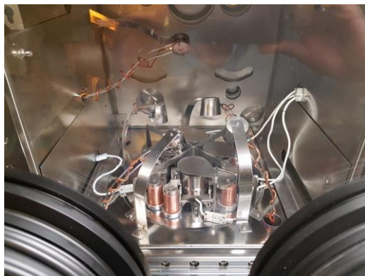
Figure 3.1. Picture of the evaporation chamber employed for the deposition of perovskite thin-films.
