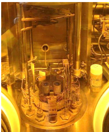
Figure 4.1. Picture of the vacuum chamber employed for the deposition of the MAPI perovskite films.
