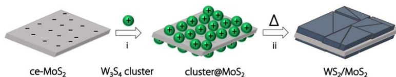
Figure V-2. Pictorial representation of WS 2 /MoS 2 synthesis: i) Synthesis of cluster@MoS 2 ; ii) Calcination of cluster@MoS 2 to give rise to the final heterostructure formed by MoS 2 layers in between WS 2 flakes (WS 2 /MoS 2 ).
